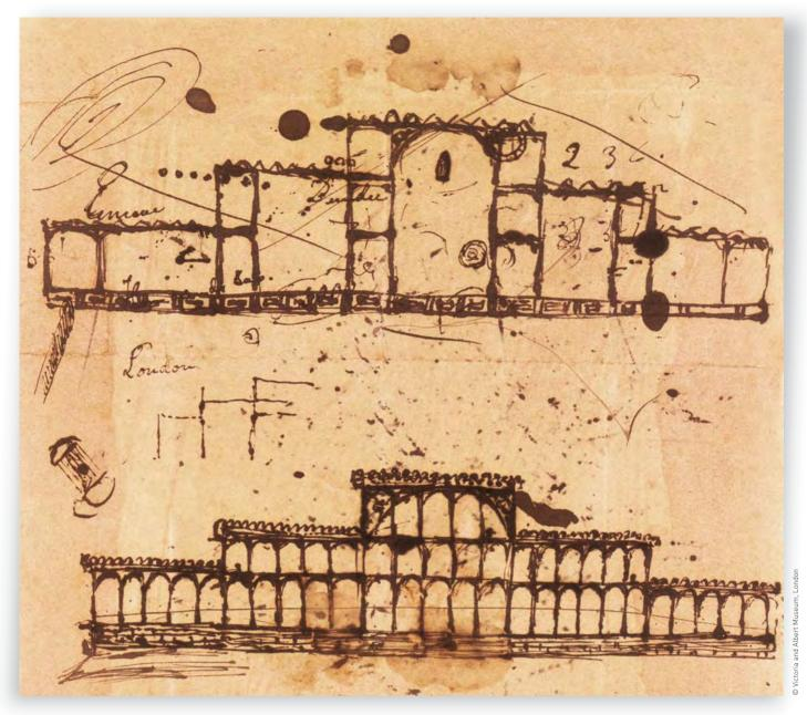
Joseph Paxton's early sketch of the Crystal Palace, drawn on pink blotting paper and showing side elevation and cross section.
