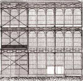
The external facade of the Crystal Palace contained approximately 300,000 glass sheets supported by over 3,000 cast-iron columns.
