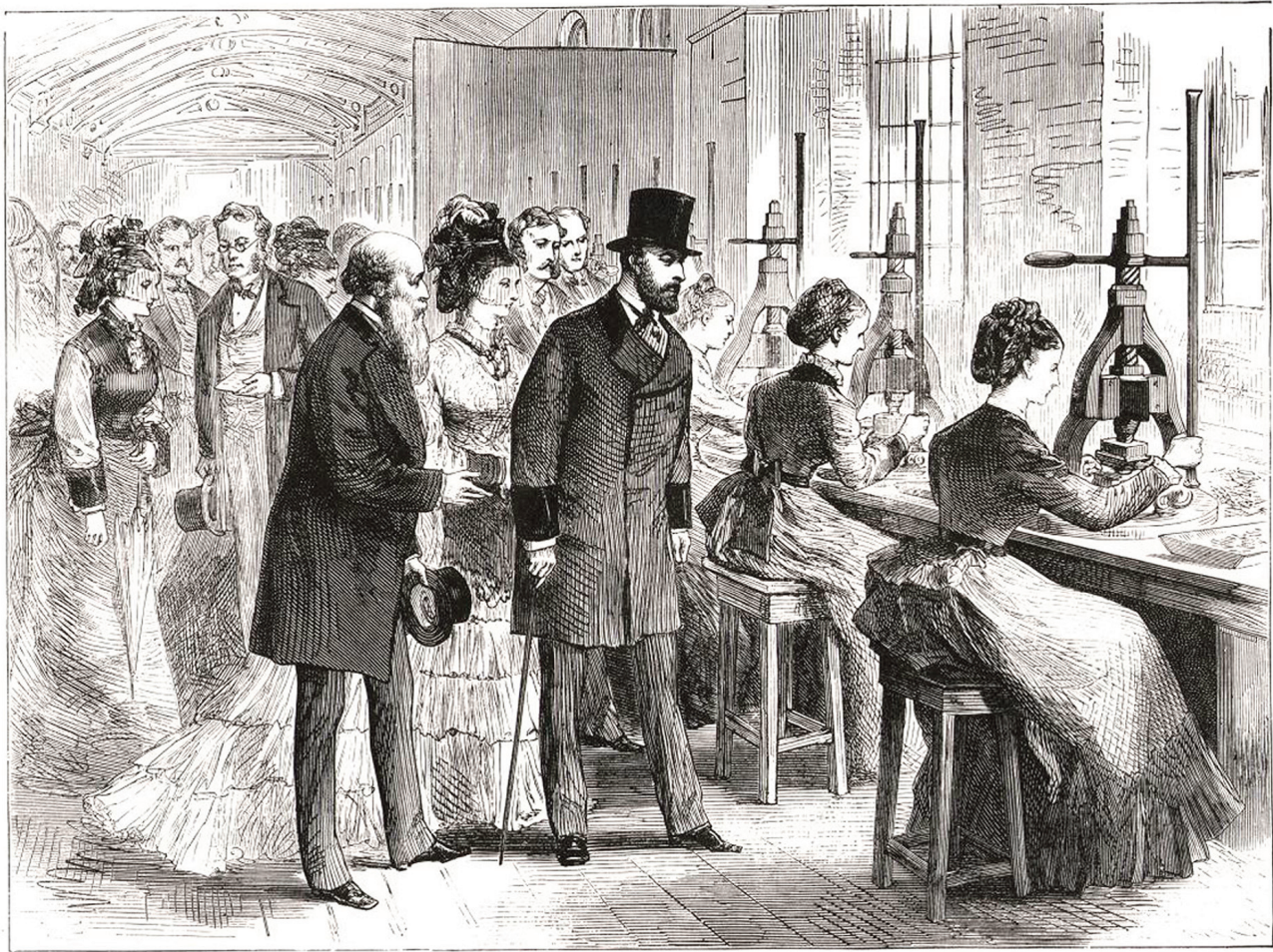
THE PRINCE AND PRINCESS OF WALES AT GILLOTT'S PEN MANUFACTORY, BIRMINGHAM: THE PROCESS OF SLITTING.
